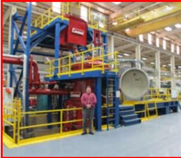
EMCC (ElectroMagnetic Cold Crucible) is a process of melting metals in a segmented water-cooled copper crucible while under vacuum or controlled atmosphere using an induction coil to heat the melt.
