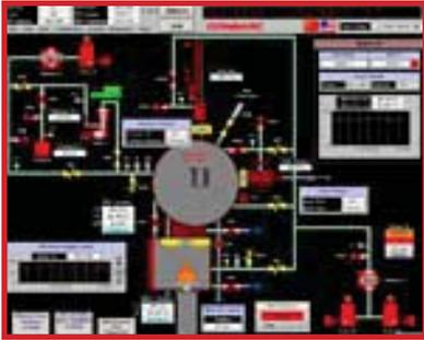
Historically, vacuum melting furnaces were essentially manually operated and it was not uncommon to have significant variances in product quality depending on the operators involved. Today, PLC and PC based supervision control systems have fully automated the VPIC furnace and operators merely have to select an appropriate 'menu' for the cast to be performed. All furnace operations can then be performed automatically, thus maintaining consistency between casts.
