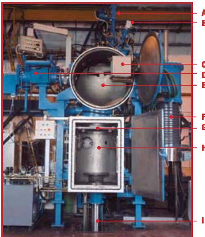
In controlled-solidification furnaces (DS and SC), in addition to the induction melting coil, the upper melting chamber contains a mold-heating zone to allow heating of the ceramic mold to temperatures above the alloy liquidus. The molds are placed on a water-cooled chill platen and withdrawn through a baffled cooling zone located directly below the heating zone. The high thermal gradient in combination with controlled withdrawal provides for controlled solidification in the cast component.
